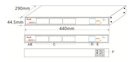
A. PWR LED Indicator C. 24\*10/100/1000M PoE Ports E.Console Port F. Power Input Port - AC100-240V,50/60Hz
